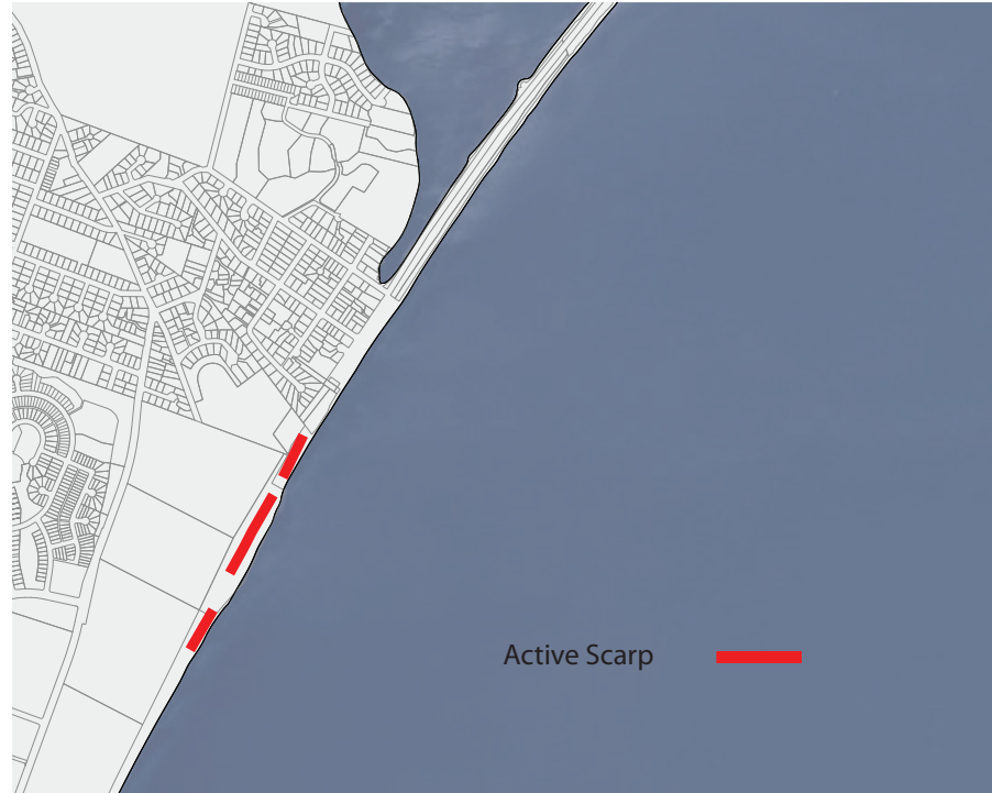
Figure 9: Current Extent of Active Scarp
