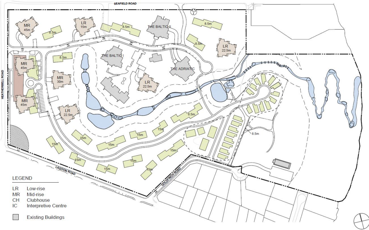
FIGURE 2 – Building heights measured from average ground level
