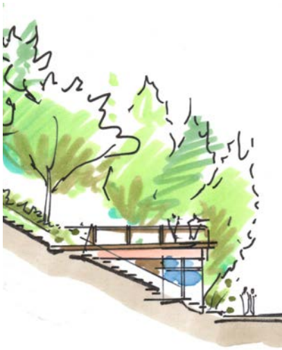
An outdoor living space is created on the roof of a building which is integrated into the topography.
