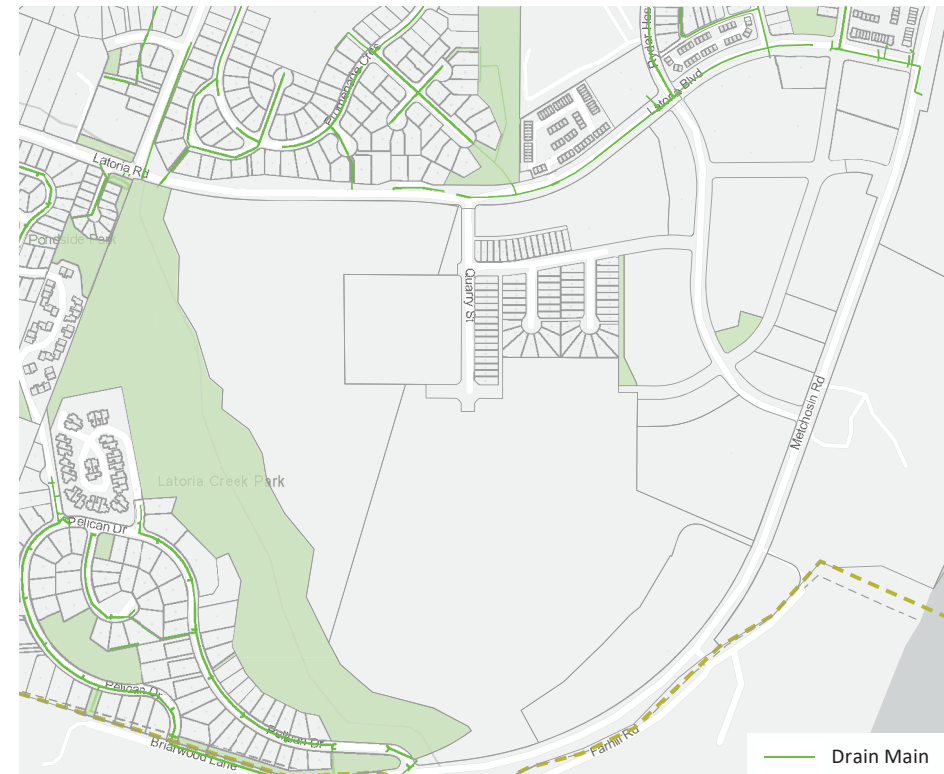
Figure 3.11 (Above): Existing Drain Main, City of Colwood GIS Mapping 2023
