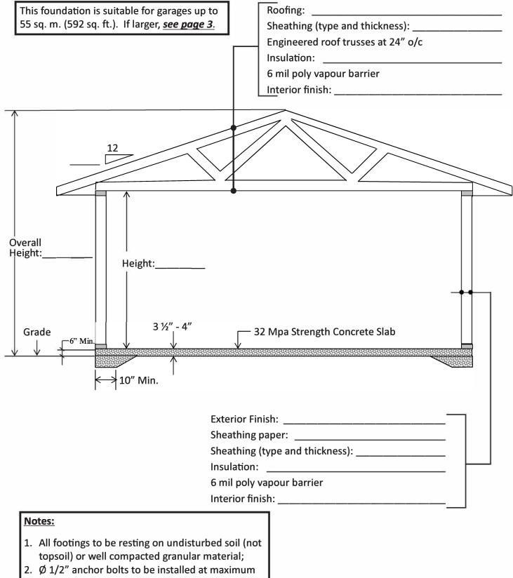
7'-10" O/C; and 3. Exterior grade to slope away from foundation.
