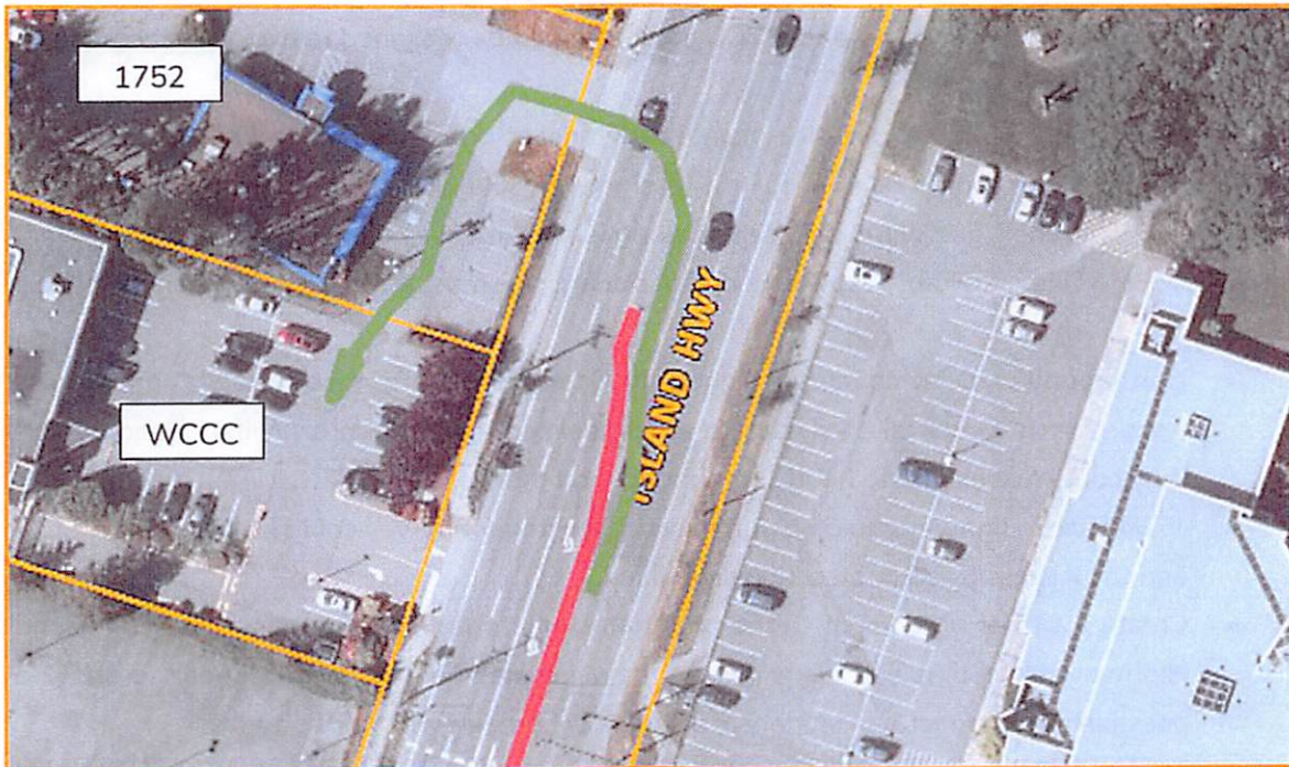
Figure 1: Existing Conditions (concrete divider in red)
