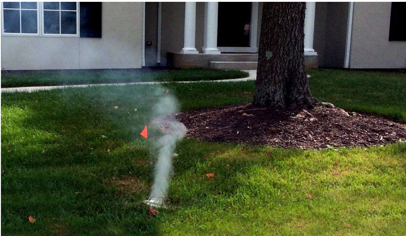
Smoke escaping from an inspection chamber (clean out) with a missing lid.
