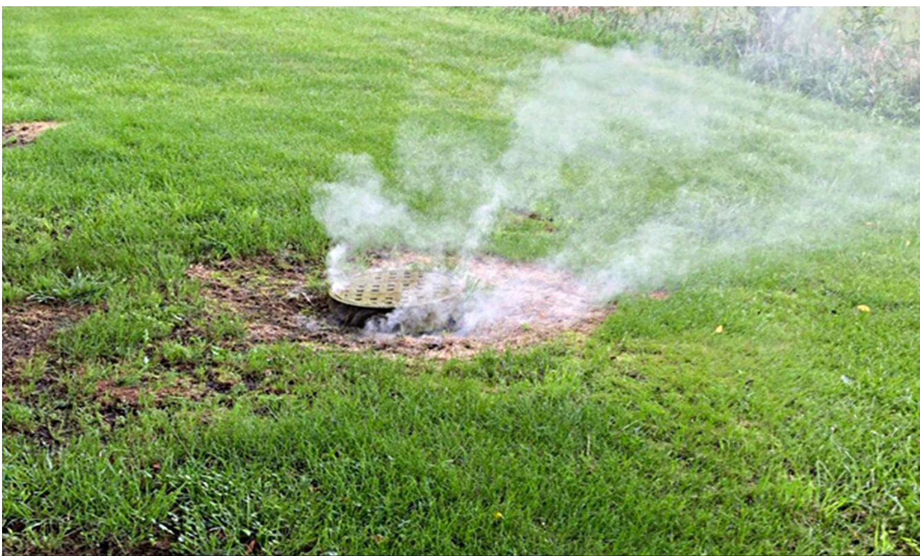
Smoke escaping from a manhole lid in an easement (sewer right of way)
