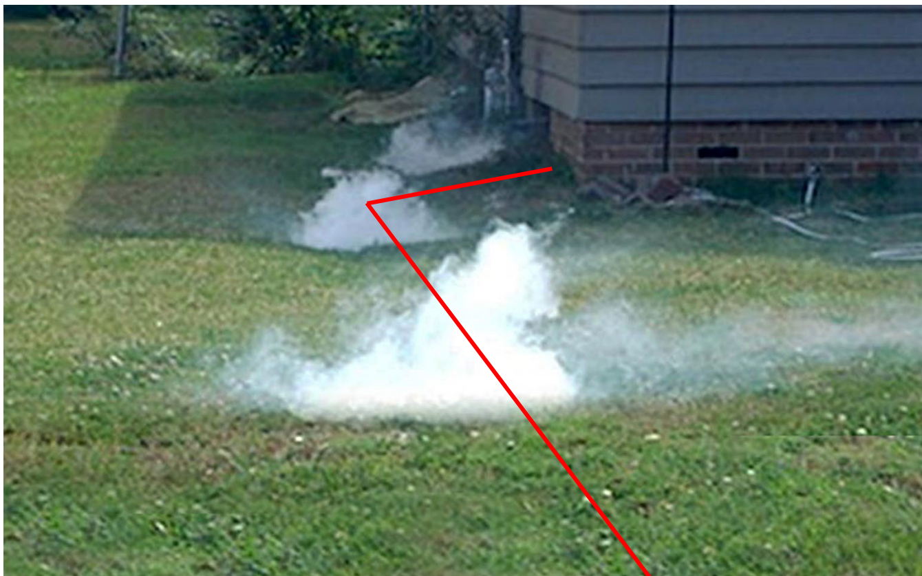
Two leaking joints on the sewer lateral (red line) leading to the house.
