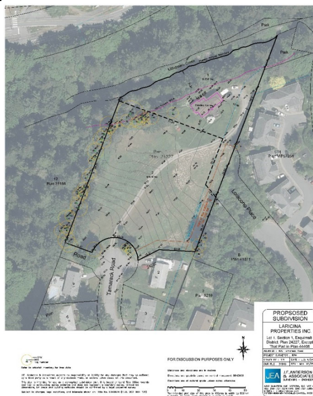
Figure 2: JE Anderson & Assoc. July 4, 2024 survey plan; mid-lot dashed black line subdivided Lot 1, 2 boundary.
