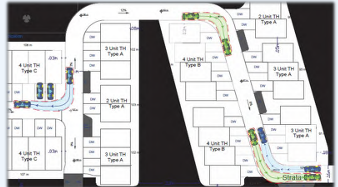
Figure 17. Vehicle Access Swept Path Analysis
